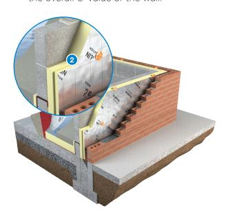
**3.** The low emissivity foil facing on the boards improves the thermal performance of the wall. The residual cavity offers an effective method of preventing wind-driven rain penetrating a wall from the outside.
