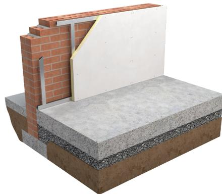
6. Seal and tape the joints of the plasterboard to ensure a continuous vapour control layer is created. Fill any gaps with foam filler or equivalent.
